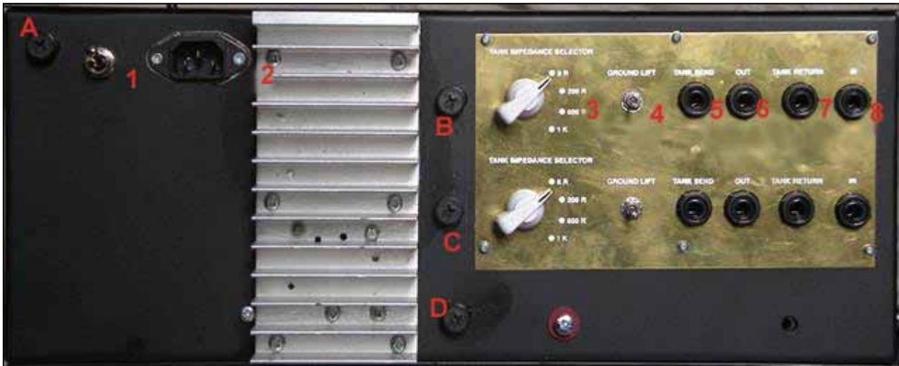
1. **Mains power switch:** in the up position, mains power is off (even if mains lead plugged in); in down position, mains power is on.
